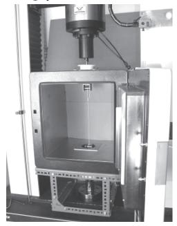
Figure 2 – Experimental set-up for tensile, TTSP and SIM test
