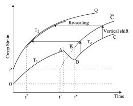
Figure 5 – Rescaling procedure for SIM
